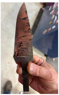
Cu Mai knives are made by welding copper into pattern welded billets. The billet was constructed in the order of 1084 steel, nickel, 1084 steel, nickel, copper, nickel, 1095 steel (3/16 inch thick for the center core) then nickel, copper, nickel, 1084 steel, nickel, 1084 steel.
